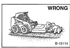
Do not put hands, feet, or objects under rotary cutter when a engine is running.
