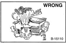
Do not use machine or rotary cutter in atmosphere with explosive dust, explosive gas, or where exhaust can contact flammable material.
